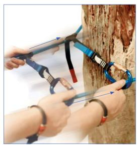
To move the STRAPLINK as close as possible to the trunk it is possible to push the prusik knot with one hand and the carabiner with the other.
