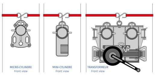
It makes it easier to position the friction device very precisely before fixing the anchoring strap(s). This way, the user needs no help to set it up.
