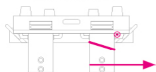
1 ROPE 3 3/4 wraps, exit right
