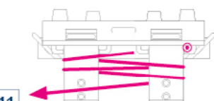
1 ROPE FIGURE-EIGHT KNOT 2 3/4 wraps, exit left
