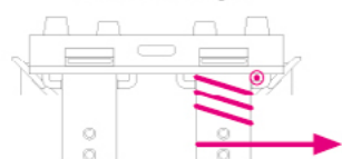
1 ROPE 3 3/4 wraps, exit right
