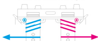
2 ROPES 3 3/4 wraps, exits left and right
