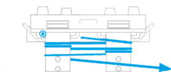
1 ROPE FIGURE-EIGHT KNOT 4 3/4 wraps, exit right
