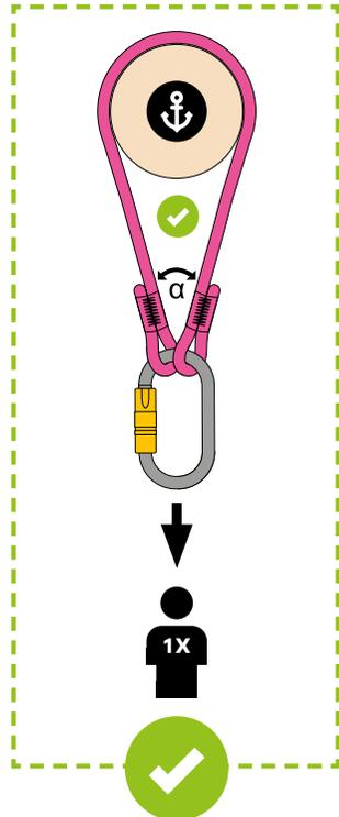
**Note :** *Single user only (100kg max.) / Maximum load angle:  $\alpha = 90^\circ$  / The maximum load that can be transmitted to the structure is approximately 8 kN / Static strength: 18 kN*
