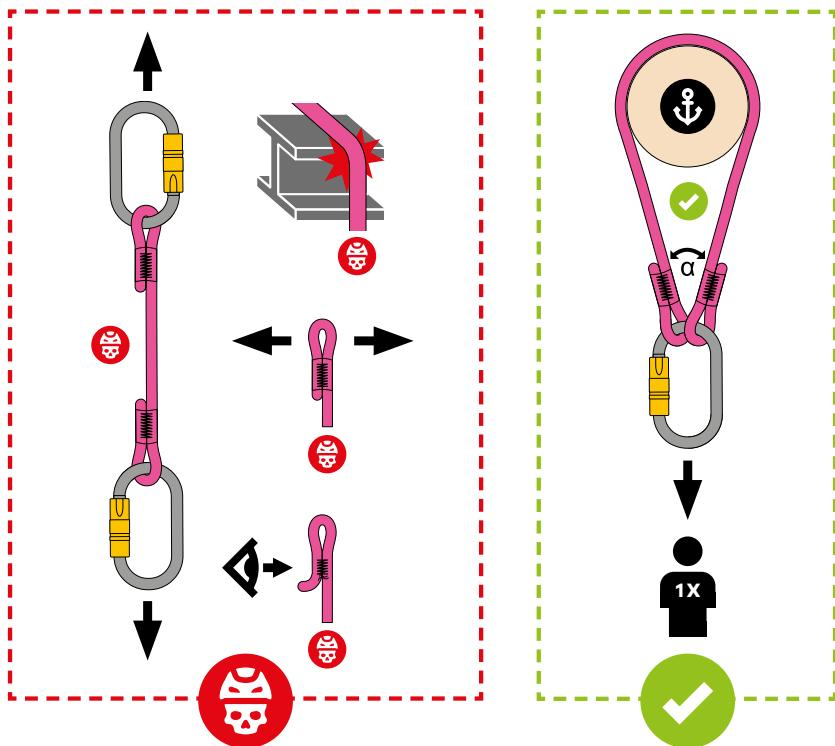
**Note:** Single user only (100 kg max.) / Maximum load angle:  $\alpha = 90^\circ$  / The maximum load that can be transmitted to the structure is approximately 8 kN / Static strength: 18 kN
